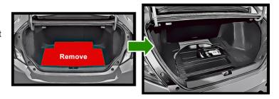
2. Remove the foam insert and set it outside the vehicle.
