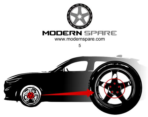
For Mach E vehicles, align the 5 lug holes directly with the spokes of the wheel.
