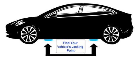
\*Please note that jacking points on vehicles may vary depending on your vehicle's make and model. Please check the user's manual if needed. Ensure to align the rubber jack pad of the scissor jack to the jacking point slot on your vehicle as shown. Failure to do so could place an uneven load on the jack resulting in jack failure.
